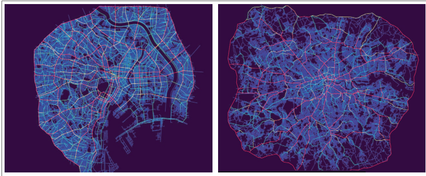
Fig. 13 Least angle choice (betweenness) analysis of Tokyo (left) and London (right) showing the network pattern in both cases.
